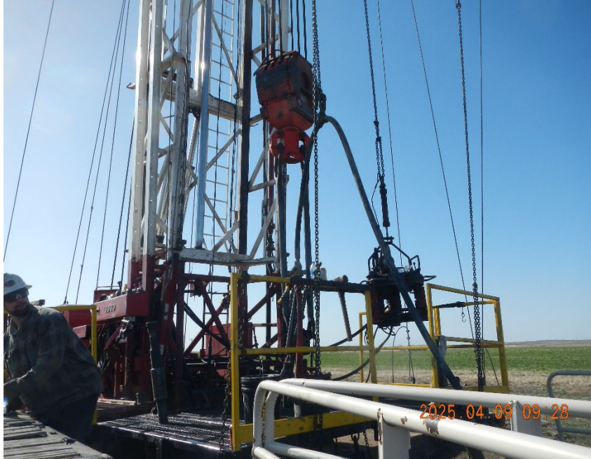
3. Pumping equipment rigged into well to pump Plug #2.
