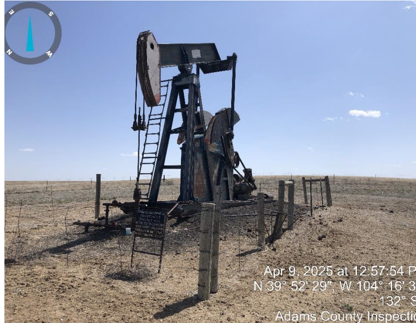
Photo #1 Pump jack.
