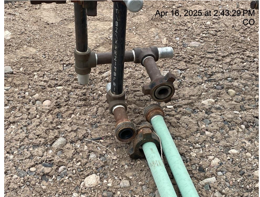
Photo # 2214 Open ended piping on the unused equipment which constitutes a wildlife hazard/available for entry by wildlife
