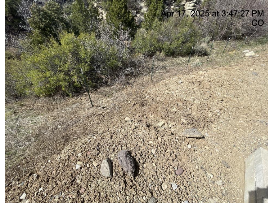
Photo # 2901 Erosion & transport of sediment off location /berm needs maintenance
