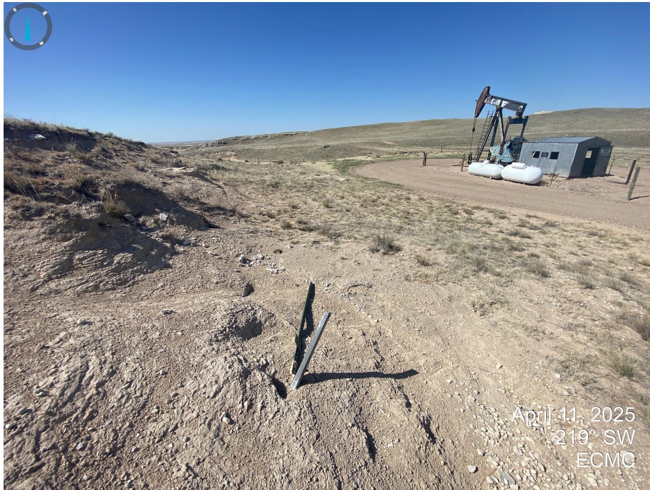
Photo 1. Northeastern guyline anchor maker needs to be reinstalled.
