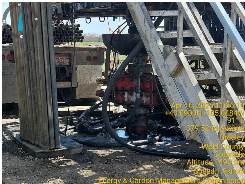
Photo 3 Wellhead/BOP.
