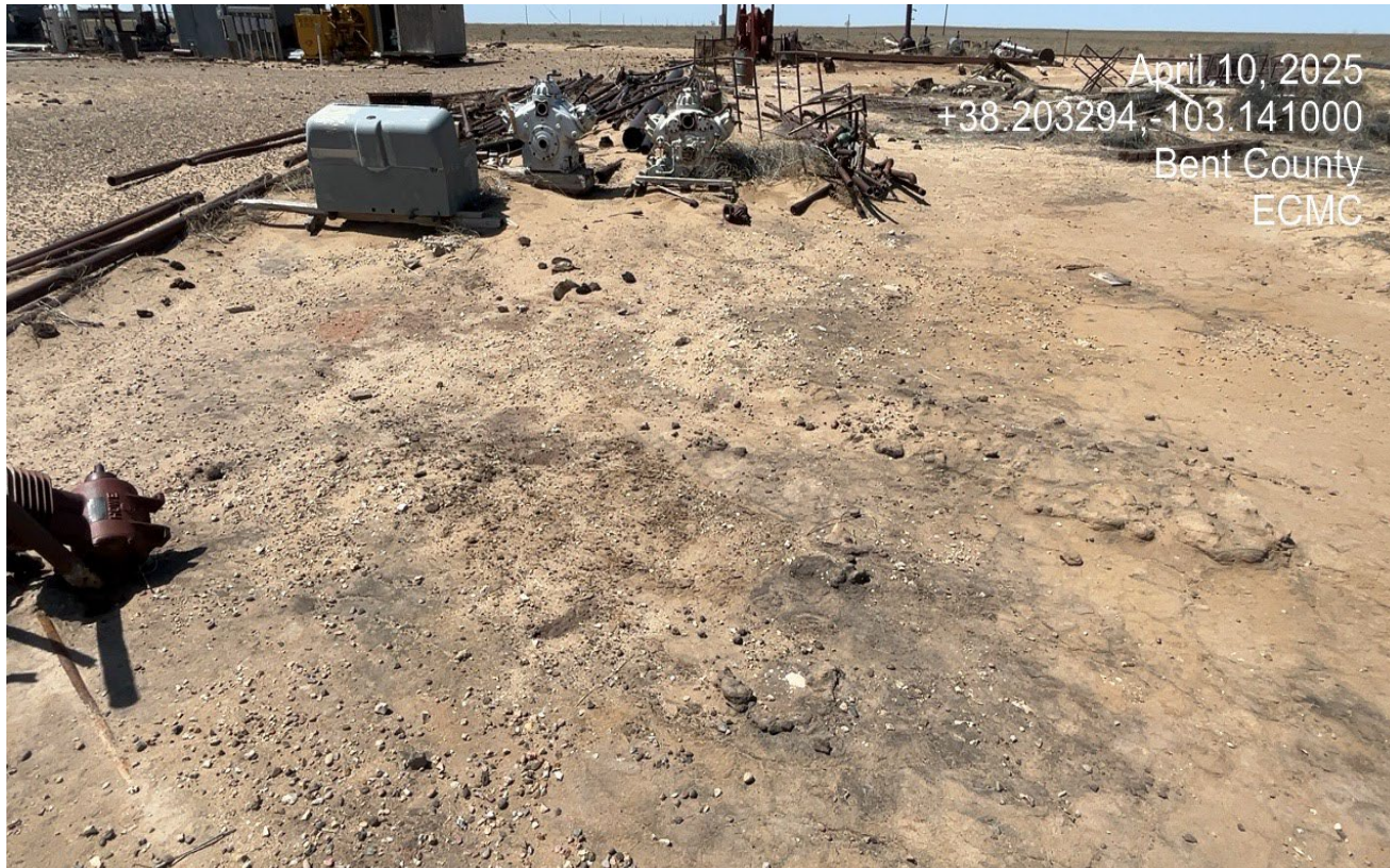
Photo 13. Facing west at the location. There is various unused equipment, supplies and tanks stored at the location that will need to be removed. The soils in this area are stained with hydrocarbon impacts from historic spill.
