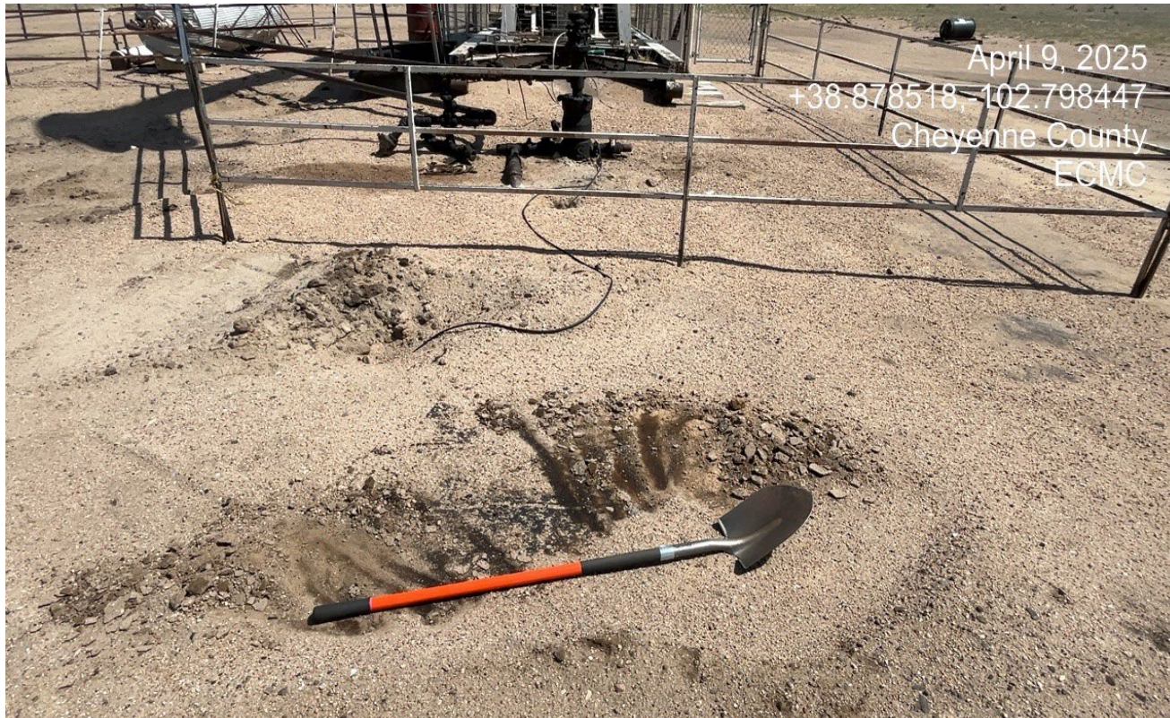
Photo 5. Closer to the well there is hydrocarbon impacts shown where shovel was placed.
