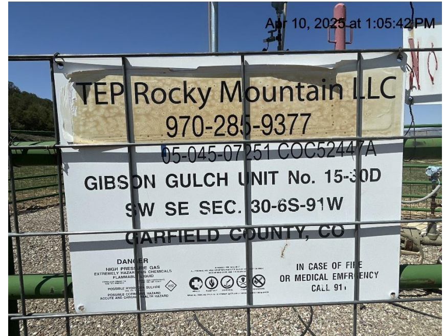
Photo # 91 Wellhead sign lacks the public road used to access the site/not in compliance with CECMC rules
