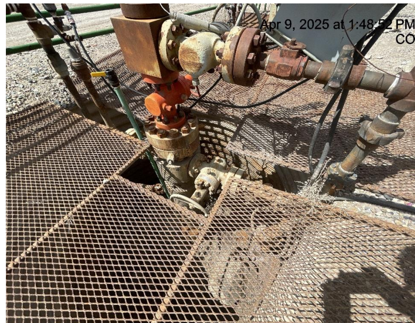
Photo # 9795 Wellhead cellar lacks wildlife egress
