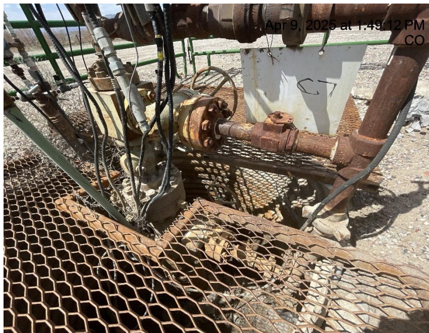
Photo # 9794 Wellhead cellar lacks wildlife egress
