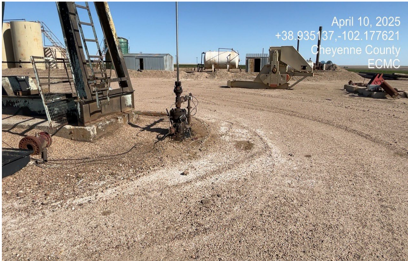
Photo 5. There is stained soils at the wellhead that need to be cleaned up and properly disposed. Also there is unused equipment stored in the upper right of the photo which needs to be removed.
