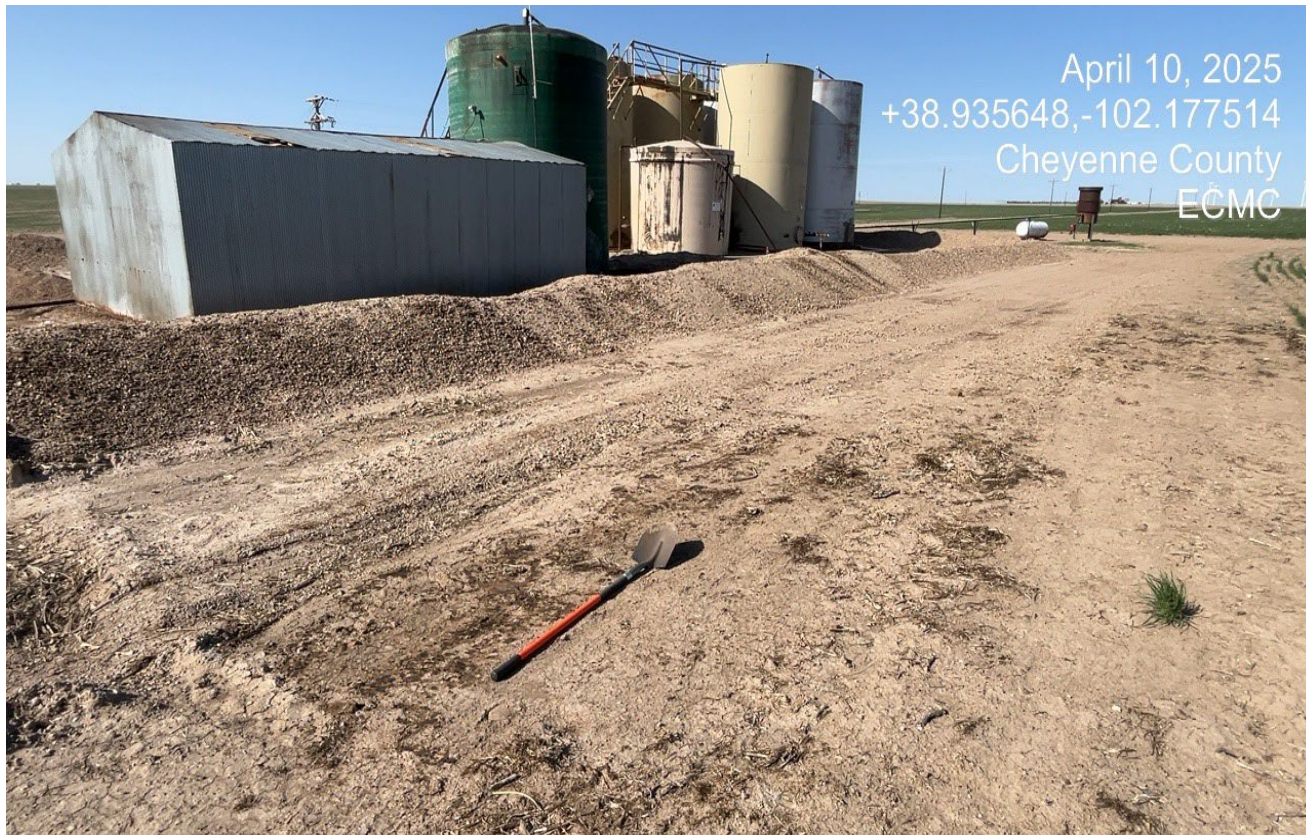
Photo 11. There is also oil stained soils that went outside of containment at the north side of the location. The shovel was placed by the stained soils for scale.
