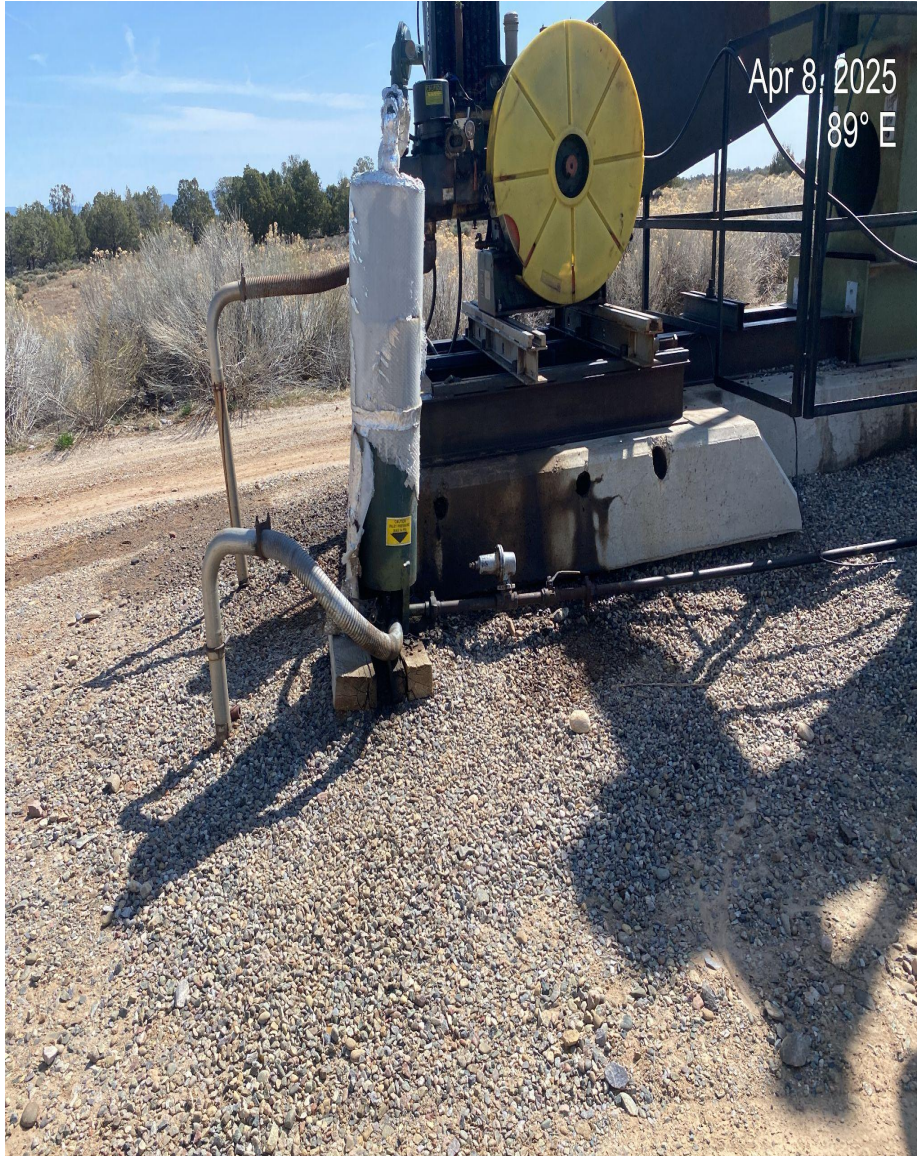
Photo 2. Stained soils at pump jacks and mufflers.
