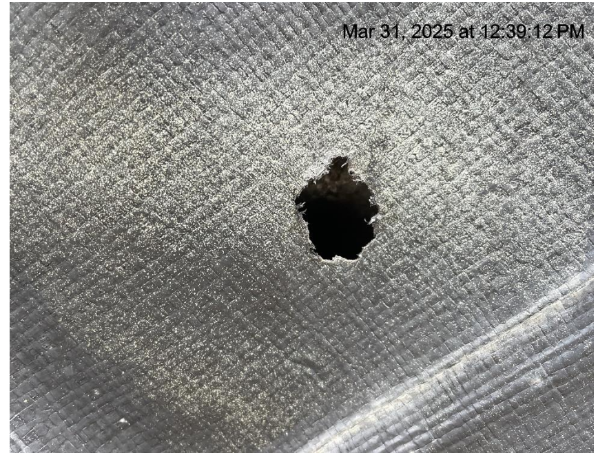
Photo # 8403 Hole in secondary containment liner/liner needs maintenance
