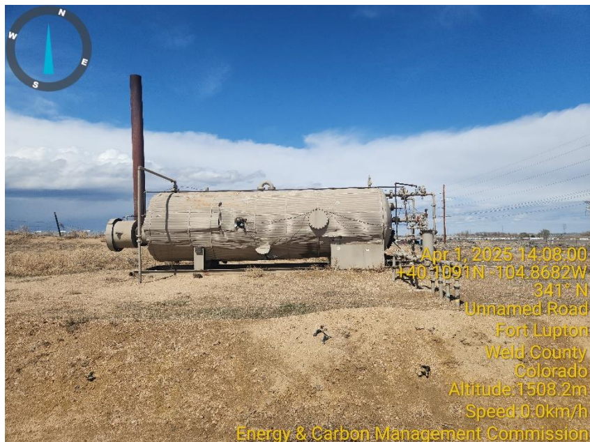
Photo 9 Horizontal Heated Separator.
