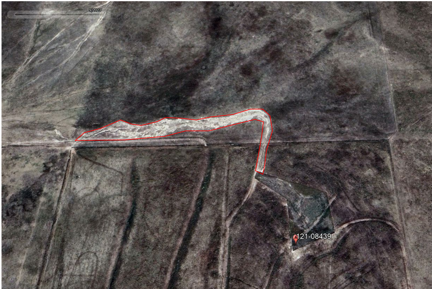
Photo 25. Google Earth aerial imagery (circa 09/2023) after facility decommissioning, illustrating salt kill impacts originating from the northwest corner of the former pit, with impacts observed throughout the adjacent drainage to the northwest/west, approximated by red outline.
