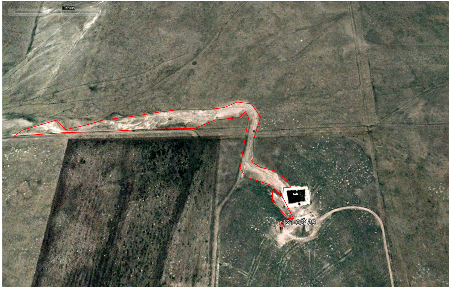
Photo 14. Google Earth aerial imagery (circa 10/2005) during active operations, illustrating salt kill impacts originating from the northwest corner of the former pit, with impacts observed throughout the adjacent drainage to the northwest/west, approximated by red outline.
