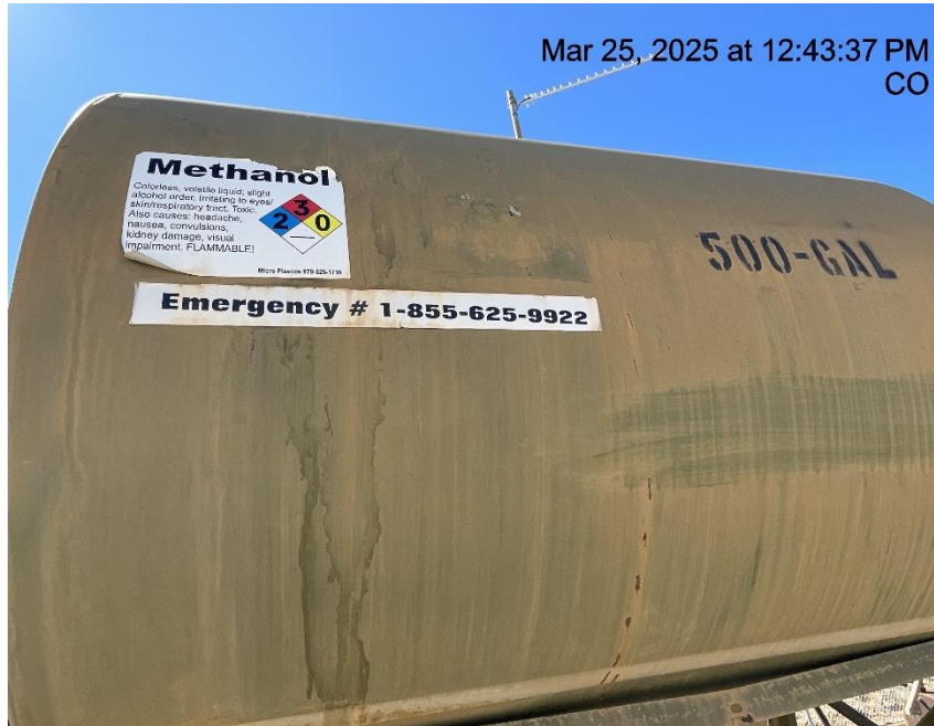
Photo # 7139 Chemical tank lacks required labeling (Additionally operator Phone # disconnected & not in service)
