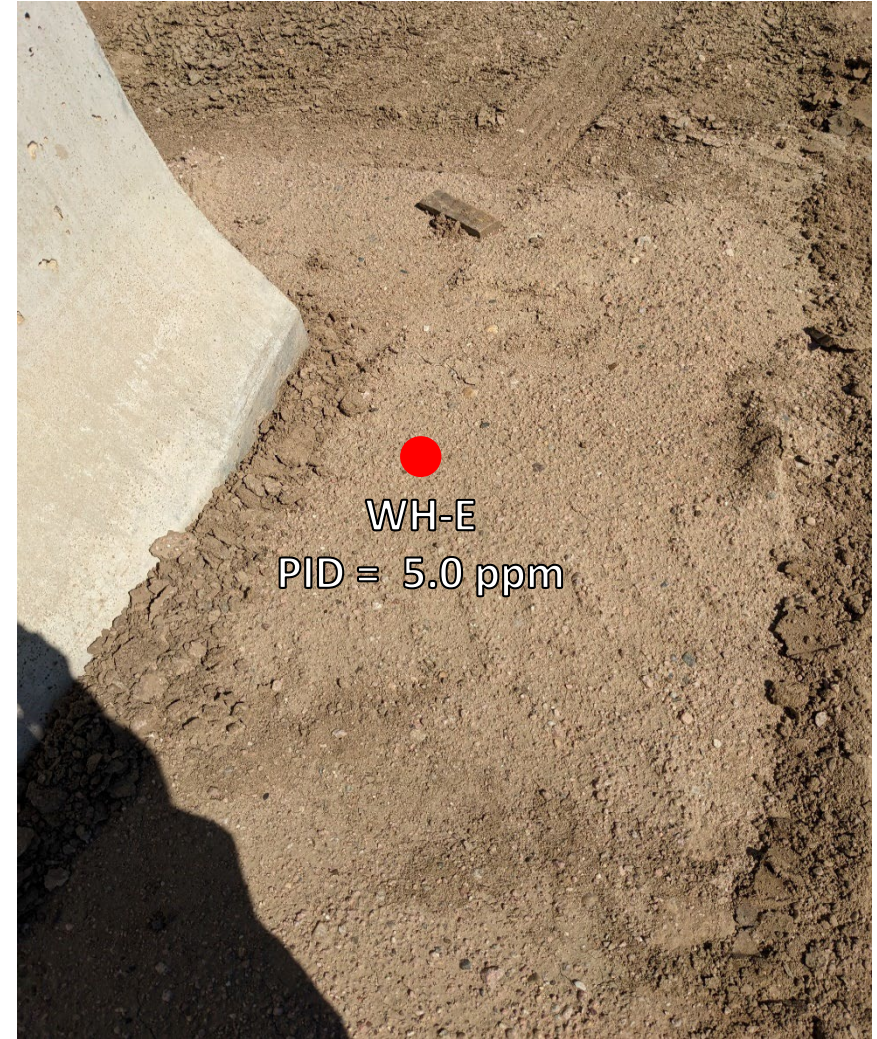
Looking east at surface screen No petroleum hydrocarbon staining or odor observed
