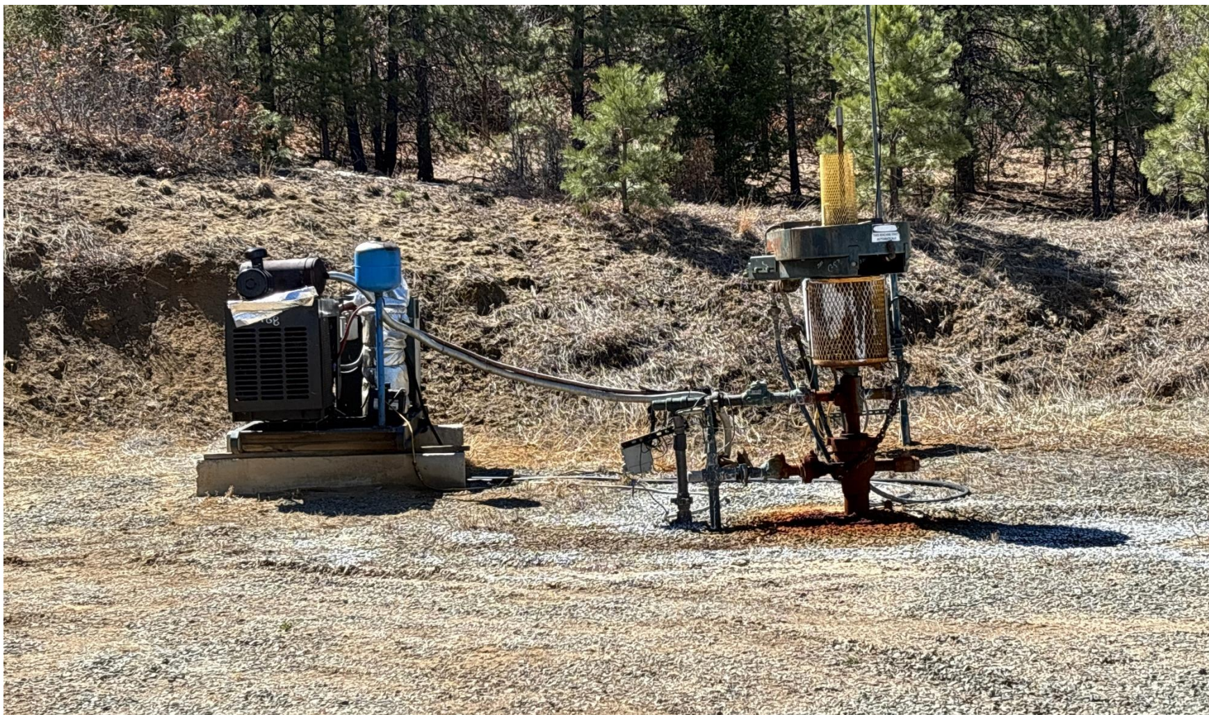
PHOTO 3: AREA OF IMPACTED SOIL AROUND WELLHEAD (SALT AND RUST COLORED IMPACTED SOIL INDICATES THAT WELL HAS BEEN LEAKING ON A REGULAR BASIS). Securely fasten all valves, pipes, fittings, and Production Facilities to ensure good mechanical condition, inspect at regular intervals, remove salt/mineral impacted soils, and maintain in good mechanical condition per Rule 608.e. CA DATE 4-2-2025.
