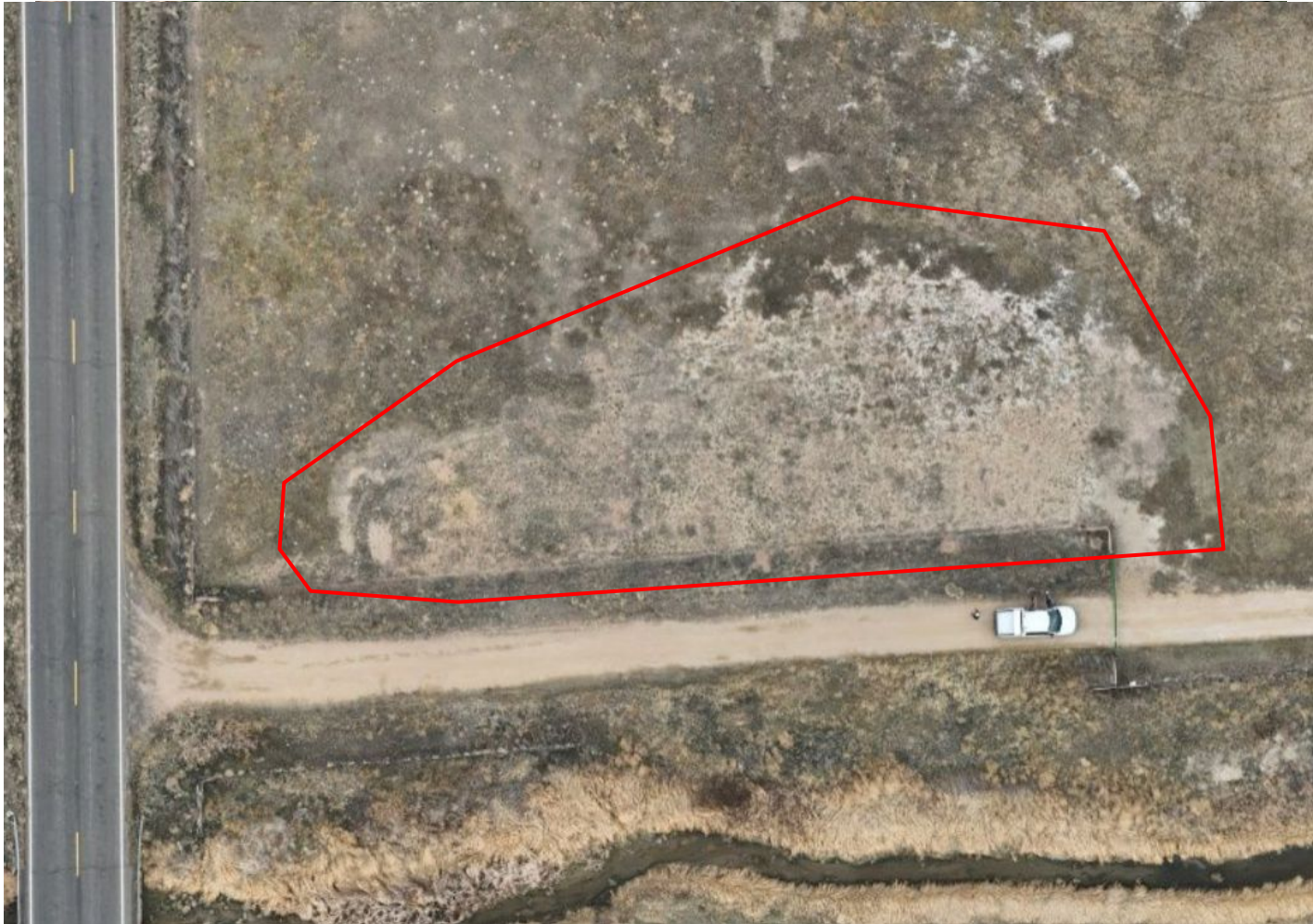
Photo 3. ECMC drone imagery taken March 25, 2025. Photo illustrates the tank battery location is evident due to the lack of vegetation establishment, which is not reflective of reference areas.
