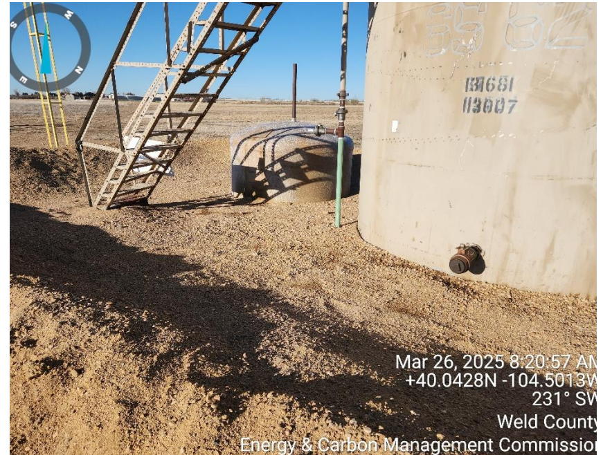
Photo 4 stained soil inside containment
