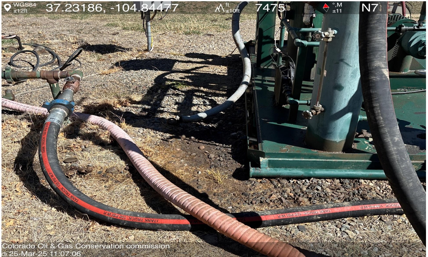
PHOTO 4: OILY WASTE NEAR COMPRESSOR. Conduct maintenance on equipment, cleanup stained material and review self inspection processes. COMPLY WITH RULE 1002,(2).D. CA DATE 3-31-2025.
