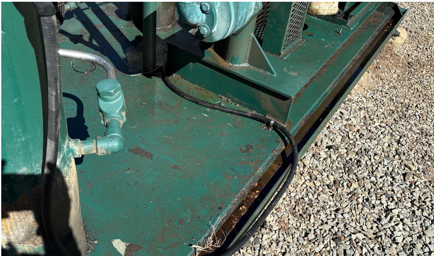
PHOTO 6: OILY WASTE IN OPEN CONTAINMENT (COMPRESSOR SKID). DRAIN OILY WASTE REPAIR ALL LEAKS AND REMOVE OR TREAT IMPACTED SOIL PER RULE 1002..(2).D & 1002.f.(2)B, Comply with general provisions of the oil and gas act for wildlife protection AND SB-181. CA DATE 3-26-2025.
