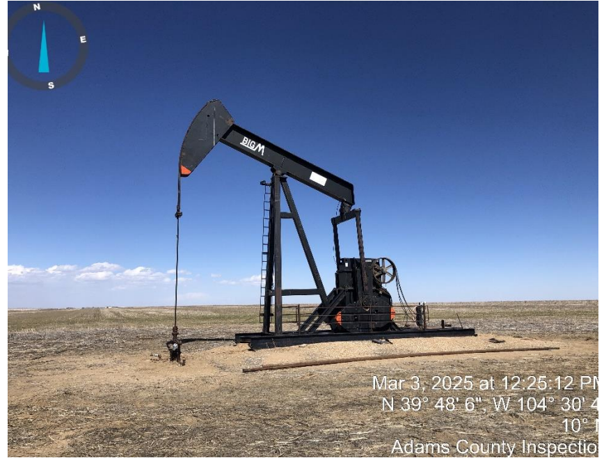
Photo #4 Pump jack.
