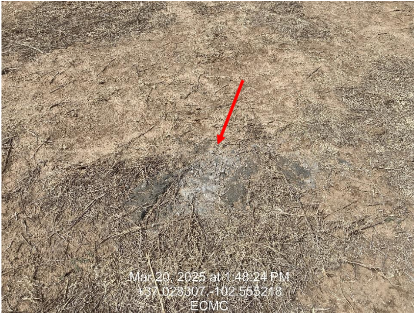
Photo 9 – Cement fines on ground east of wellhead
