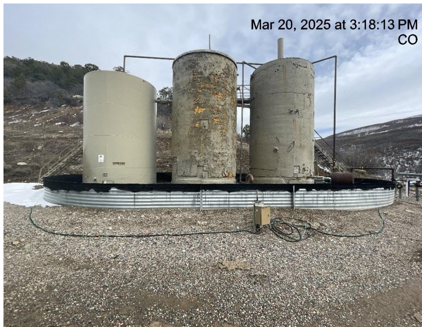
Photo # 6255 Tank battery lacks required signage
