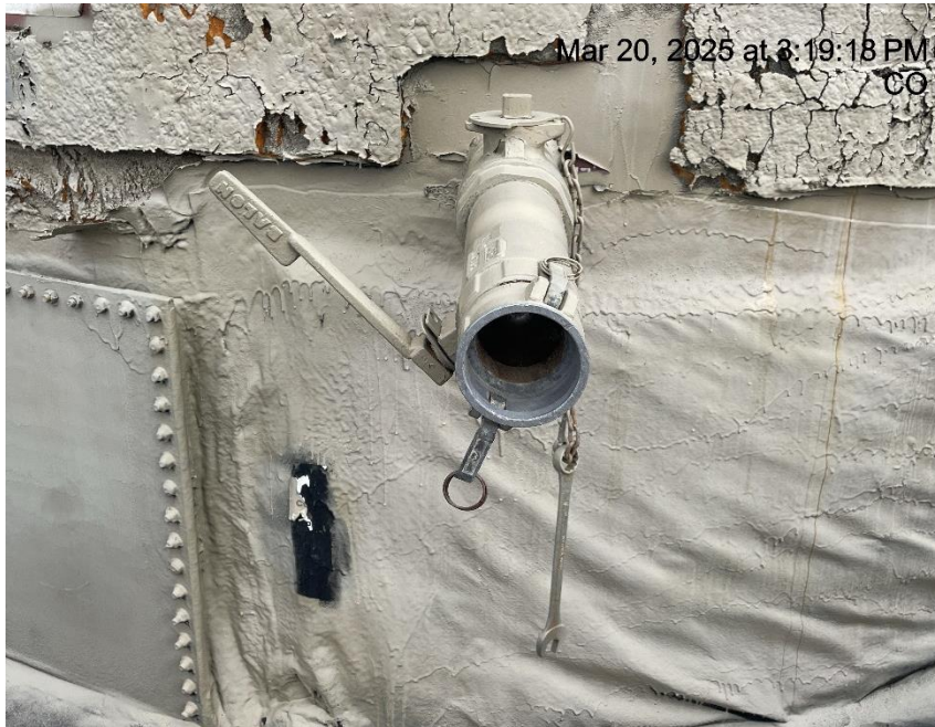
Photo # 6251 Open ended load line
