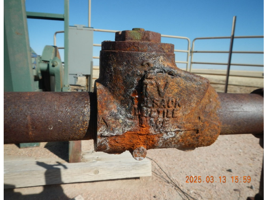
4. View of split in check valve body.
