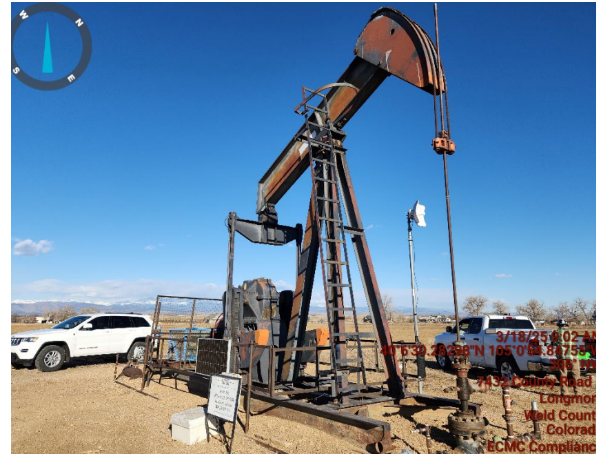
Photo 2: SI Pumpjack. Overgrown vegetation removed
