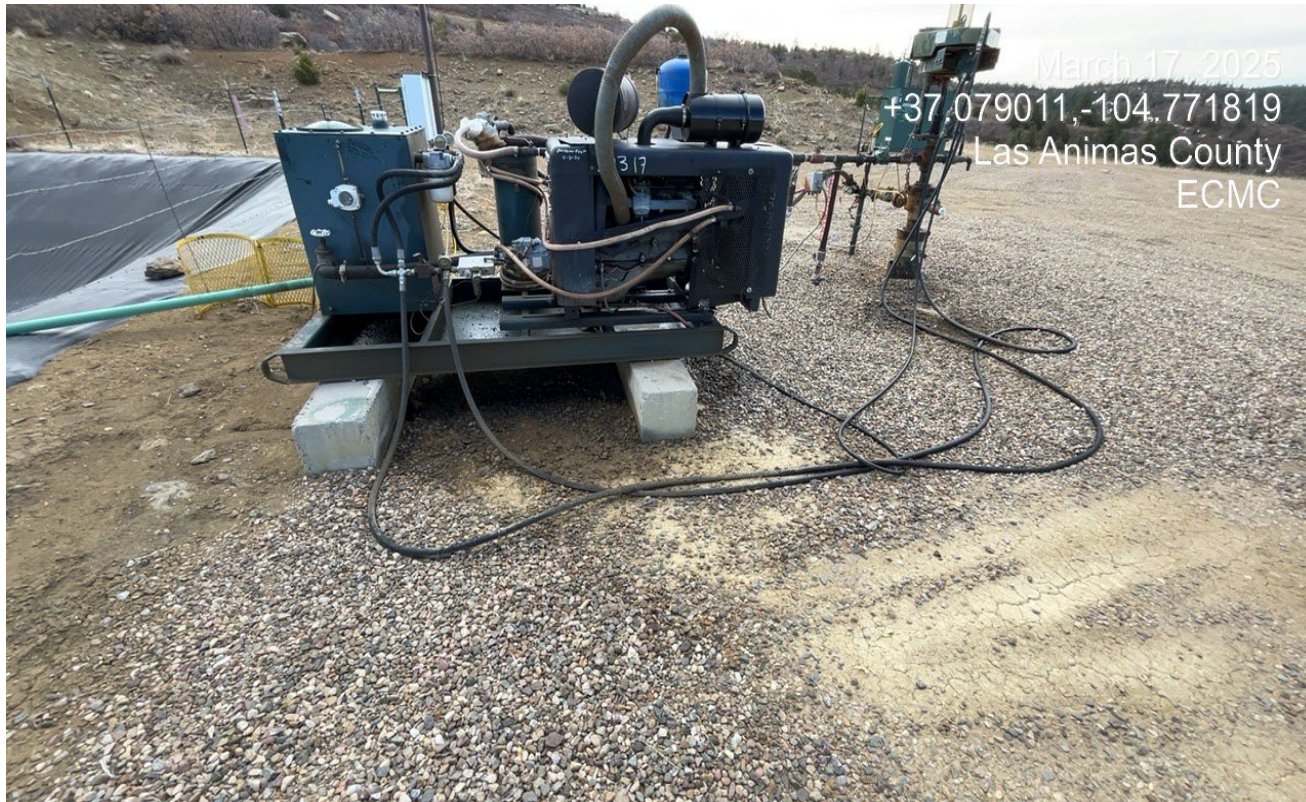
Photo 3. There is oil staining under the engine skid and at the wellhead that needs to be cleaned up.
