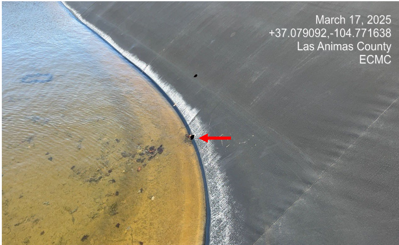
Photo 5. There are two holes in the liner and the water level is right at the first hole shown at red arrow.
