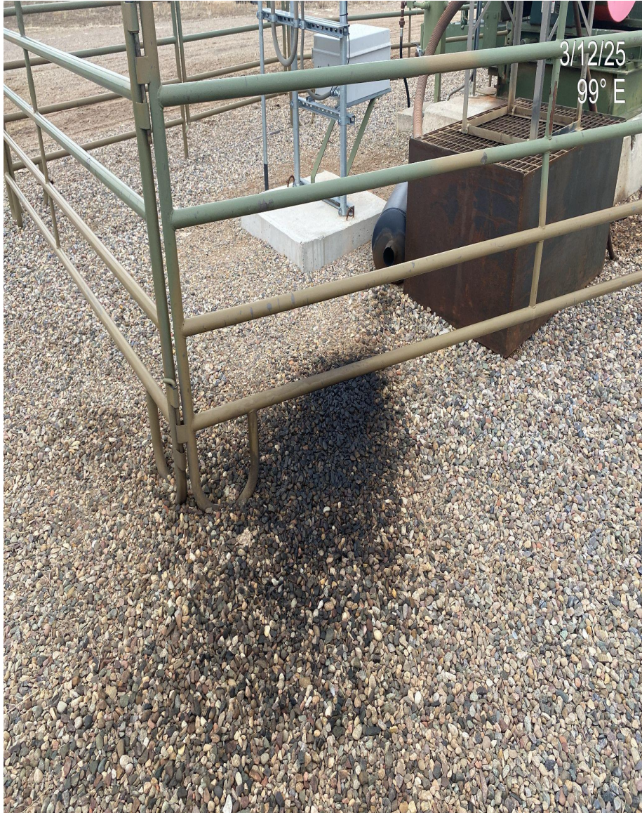
Photo 3. Stained soils at wellhead #4 muffer and pump jack platform.
