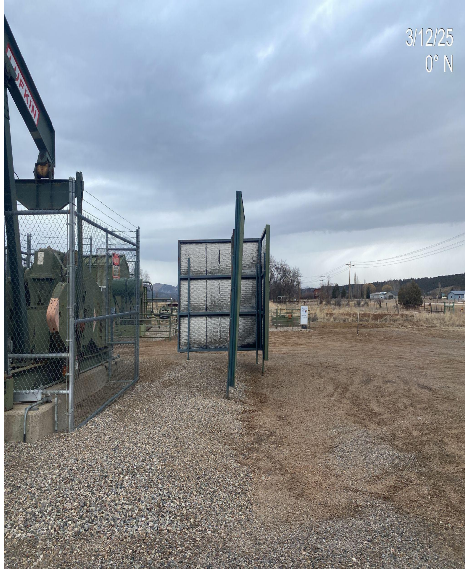
Photo 2. Sound panels have been reinstalled at the pump jack.
