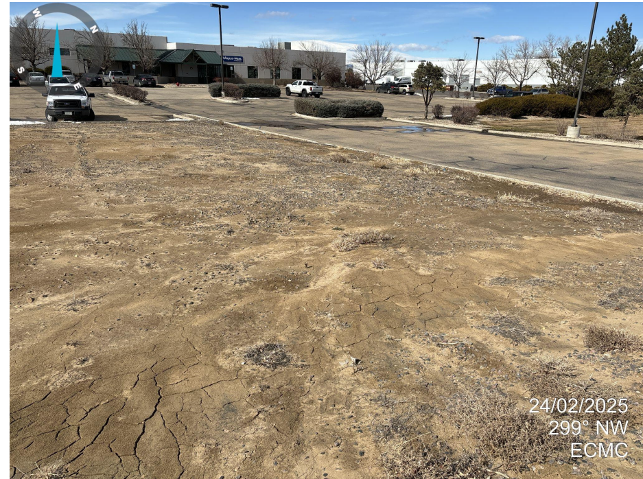
Photo 6. Looking west across location. Soil is not stabilized, erosion channels are beginning to form.
