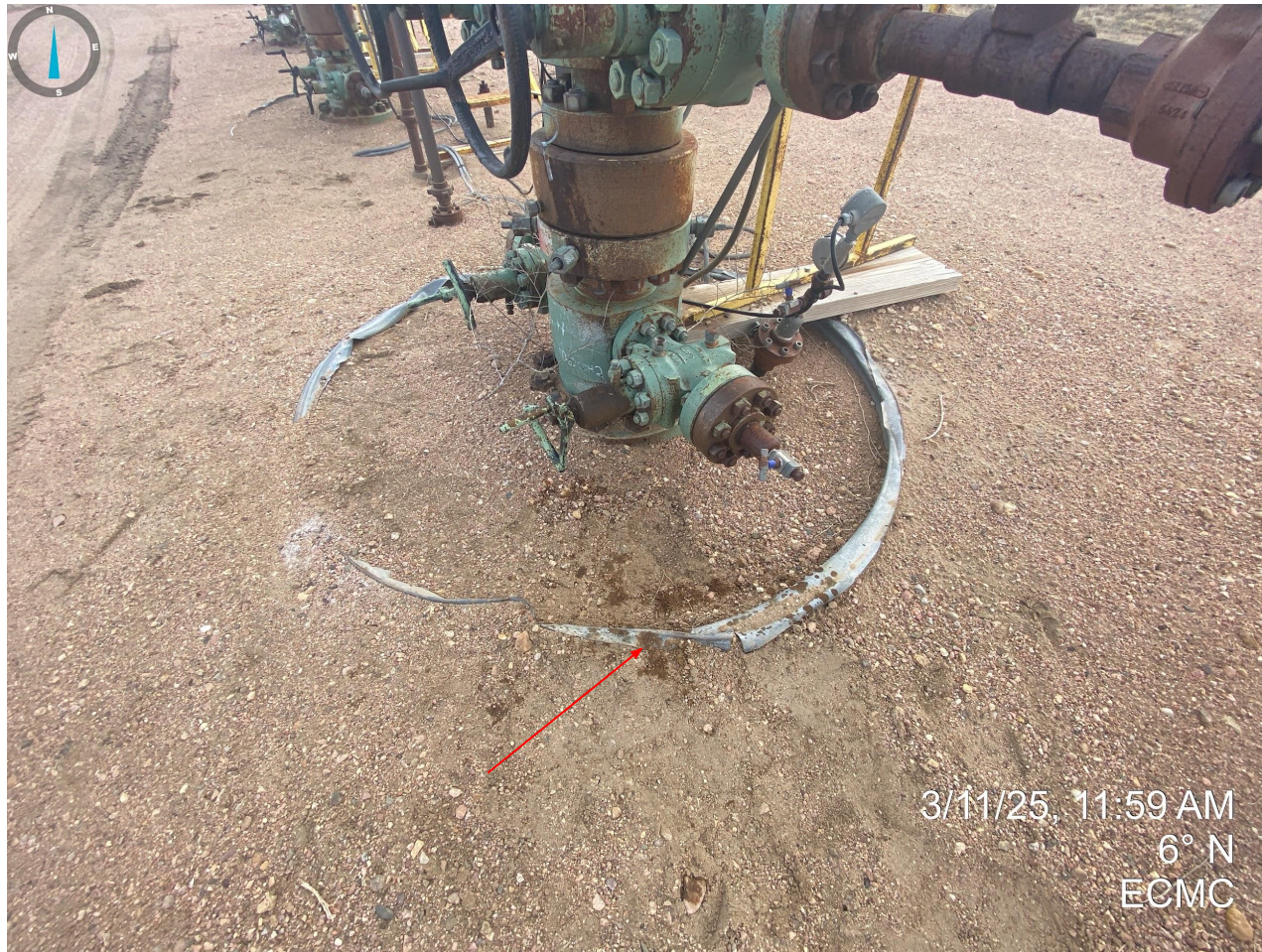
Photo 15. Hydrocarbon staining observed at wellhead.
