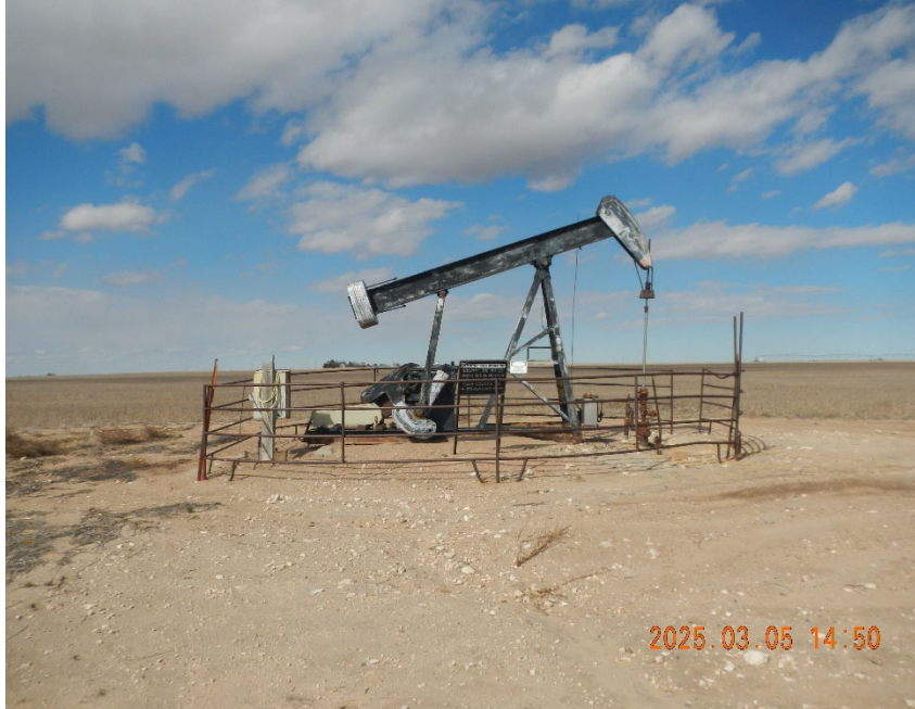
3. Looking towards well from edge of location. Note erosion channel at lower right to center of frame.
