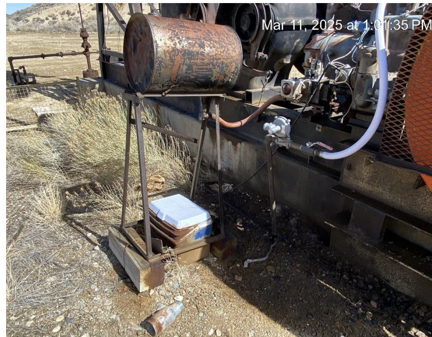
Debris. Stained soil. No containment.
