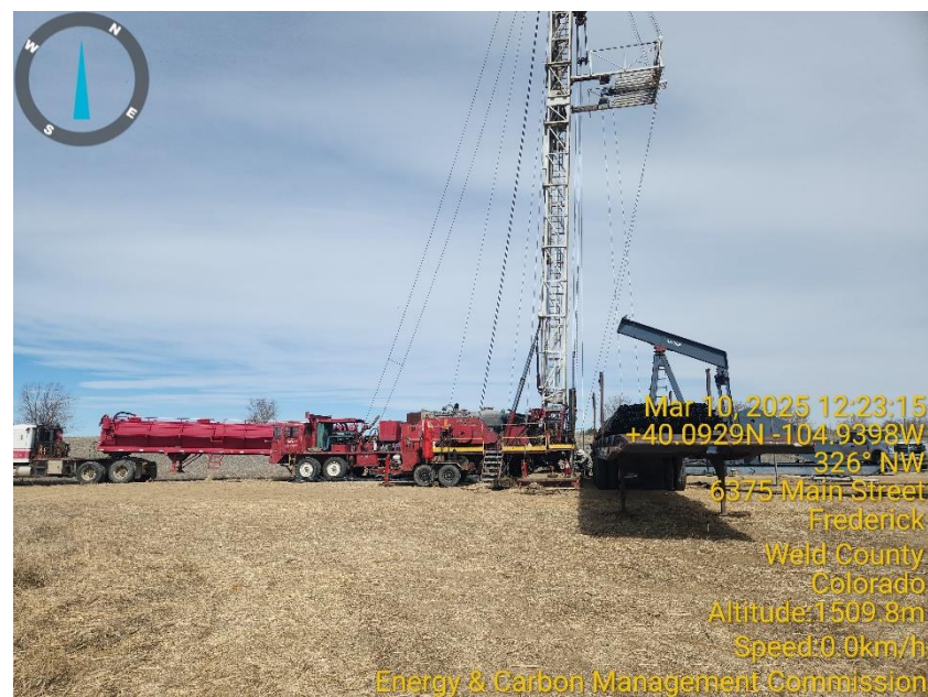
Photo 2 WO rig tubing trailer & accumulator trailer.
