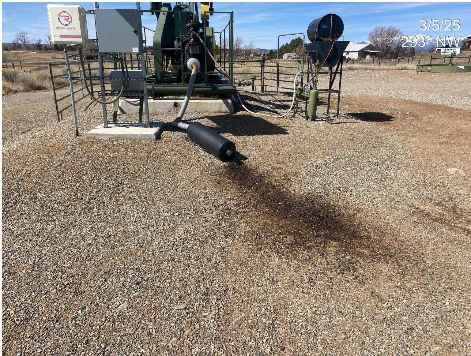
Photo 2. Stained soils at pump jack muffler.
