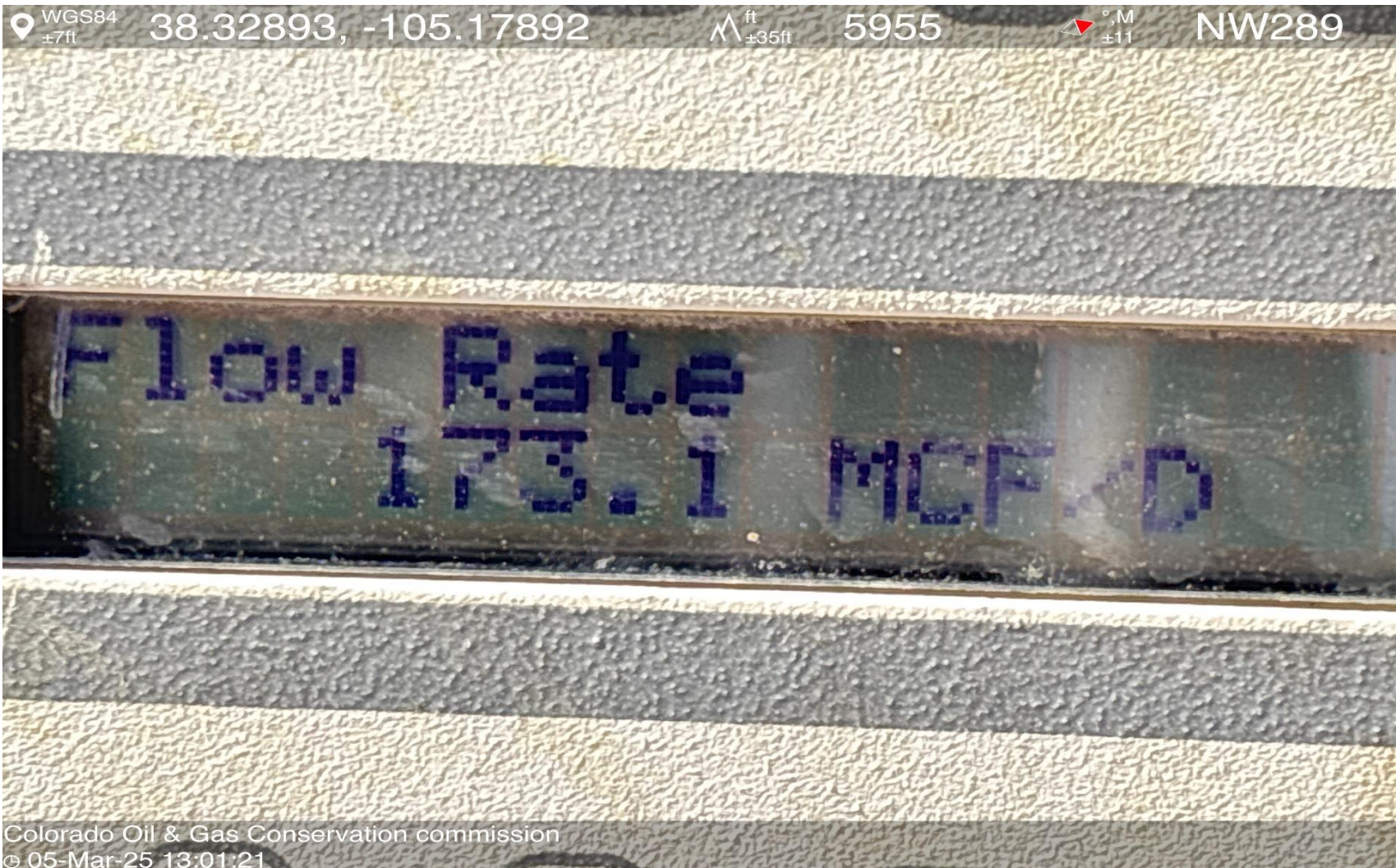
PHOTO 12: METER ONE SHOWS GAS PRODUCTION HOWEVER NO PRODUCTION HAS BEEN REPORTED BY OPERATOR. SUBMIT PRODUCTION REPORTS PER RULE.
