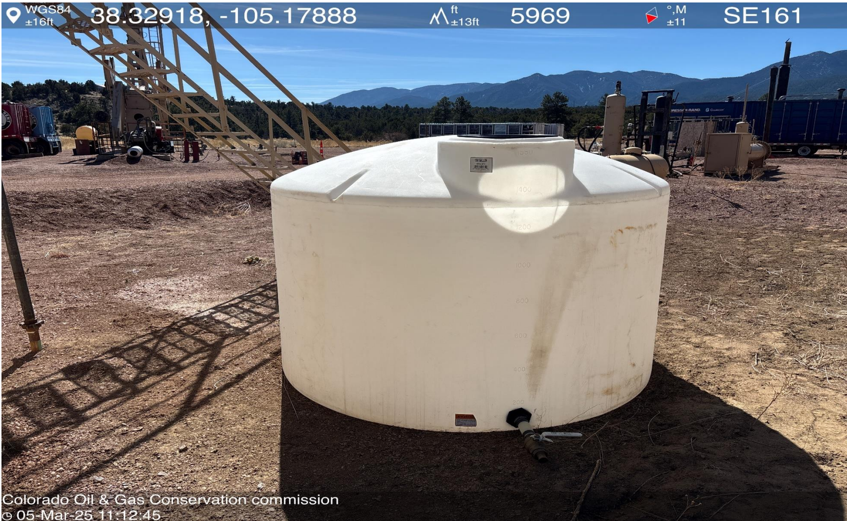
PHOTO 6: 1550 GAL TANK NEXT TO PERMANENT IS NOT LABELED. Install sign to comply with Rule 605.h. CA DATE 4/5/2025.
