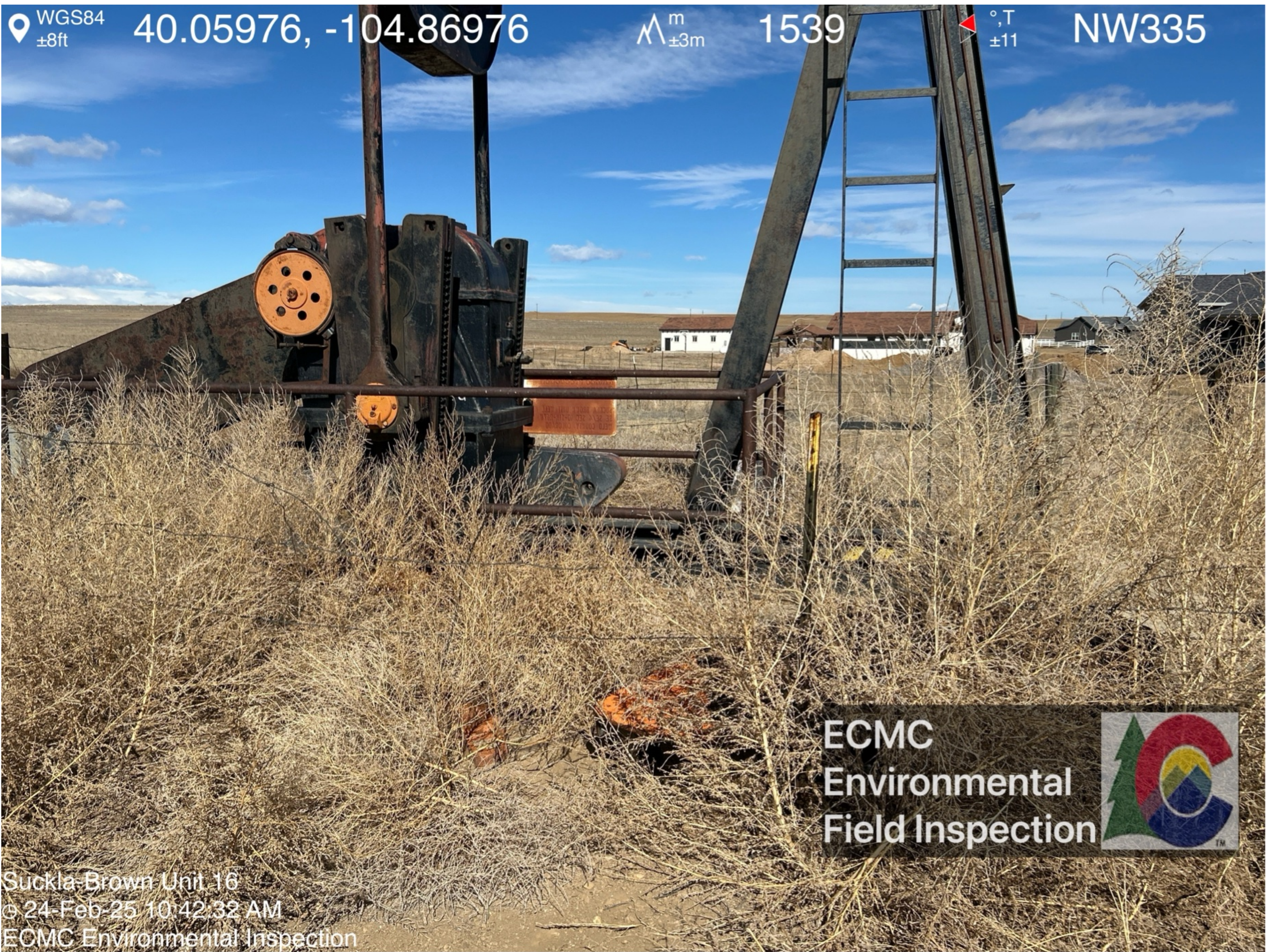
Pumping unit components visible on the ground surface adjacent to the wellhead.
