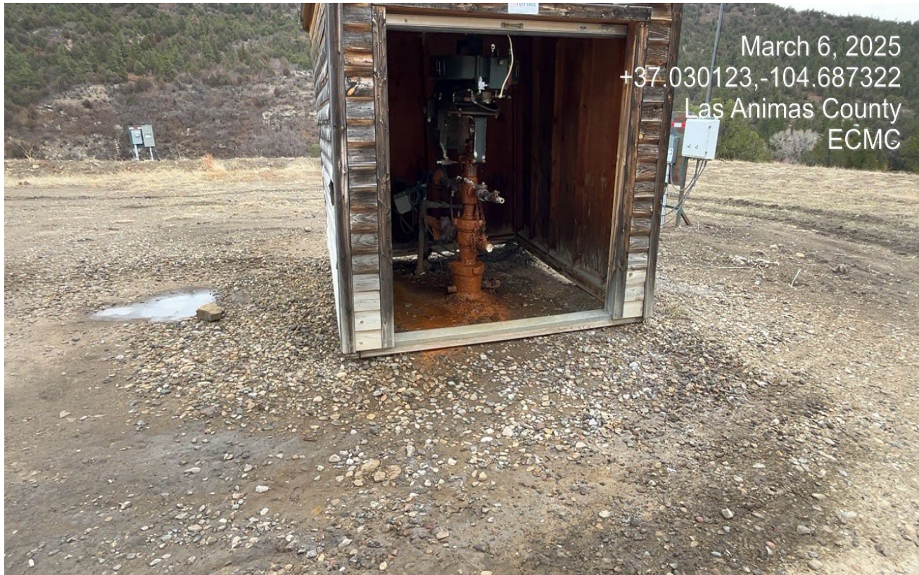
Photo 4. There is a dripping water leak at the wellhead.
