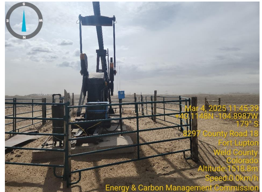
Photo 4 Prime mover is a gas engine.
