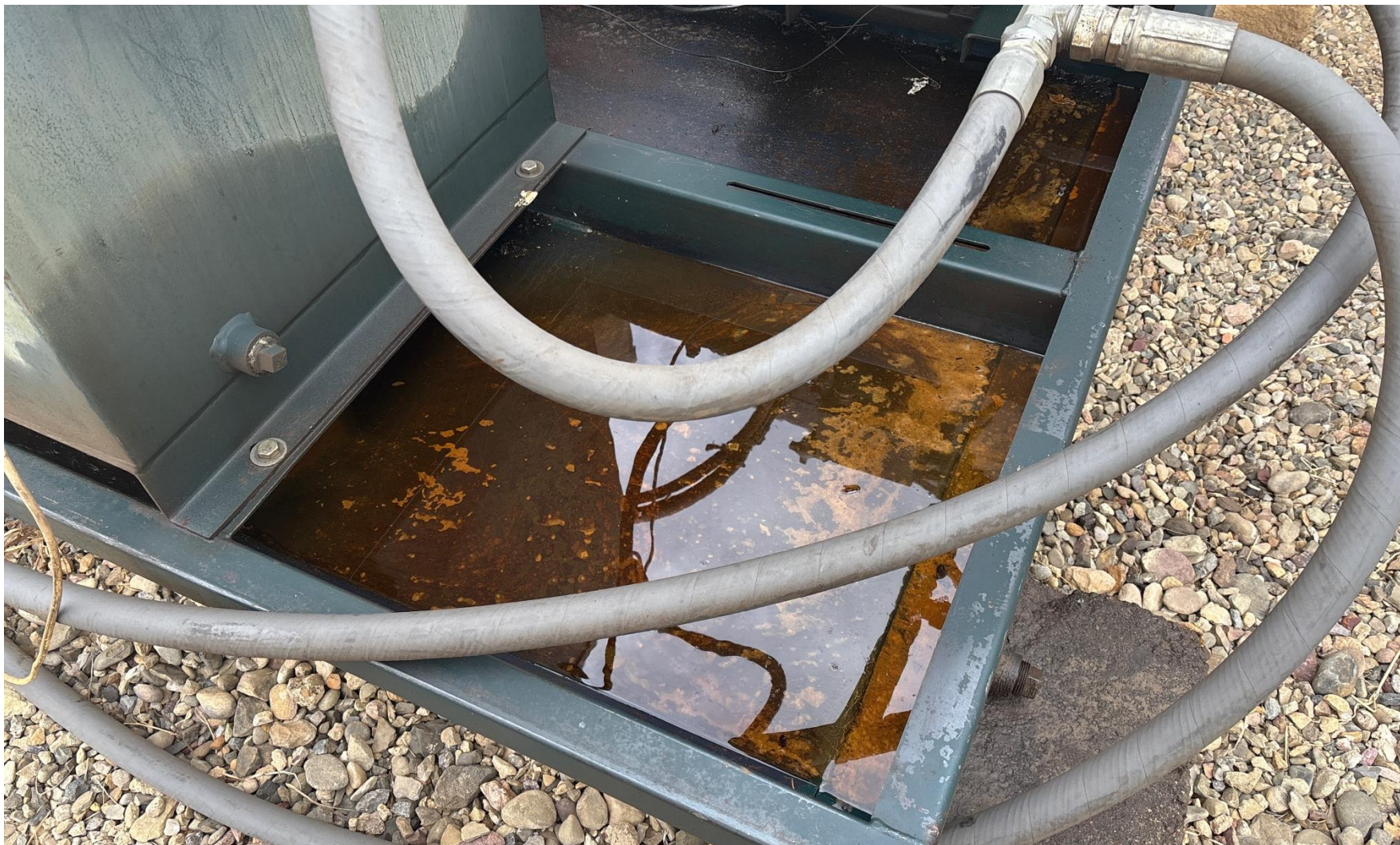
PHOTO 4: OILY WASTE IN PRIME MOVER ENGINE SKID. DRAIN OILY WASTE REPAIR ALL LEAKS AND REMOVE OR TREAT IMPACTED SOIL PER RULE 1002..(2).D & 1002.f.(2)B, Comply with general provisions of the oil and gas act for wildlife protection AND SB-181. CA DATE 3/4/2025.
