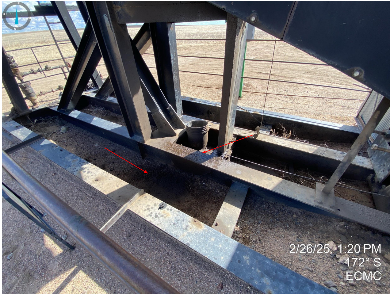
Photo 8. Stained soil observed at pumpjack unit.
