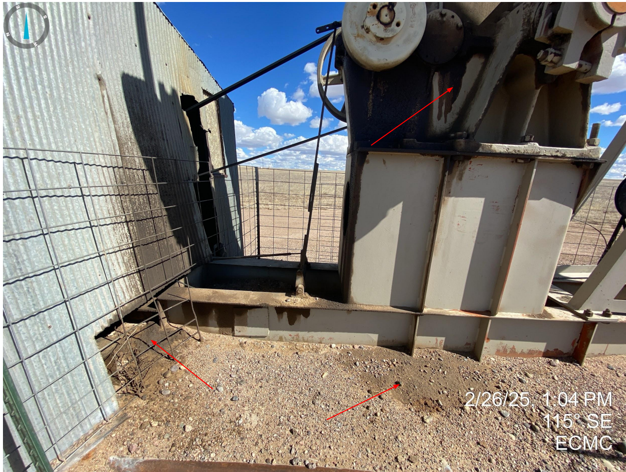
Photo 3. Stained soil and leaking equipment at pumpjack unit.
