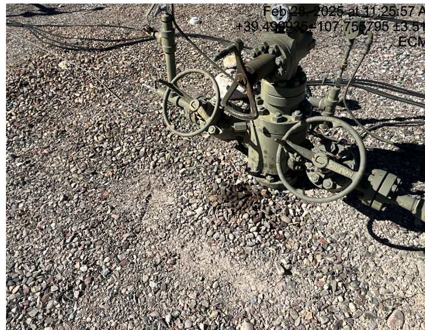
Staining (master valve grease)
