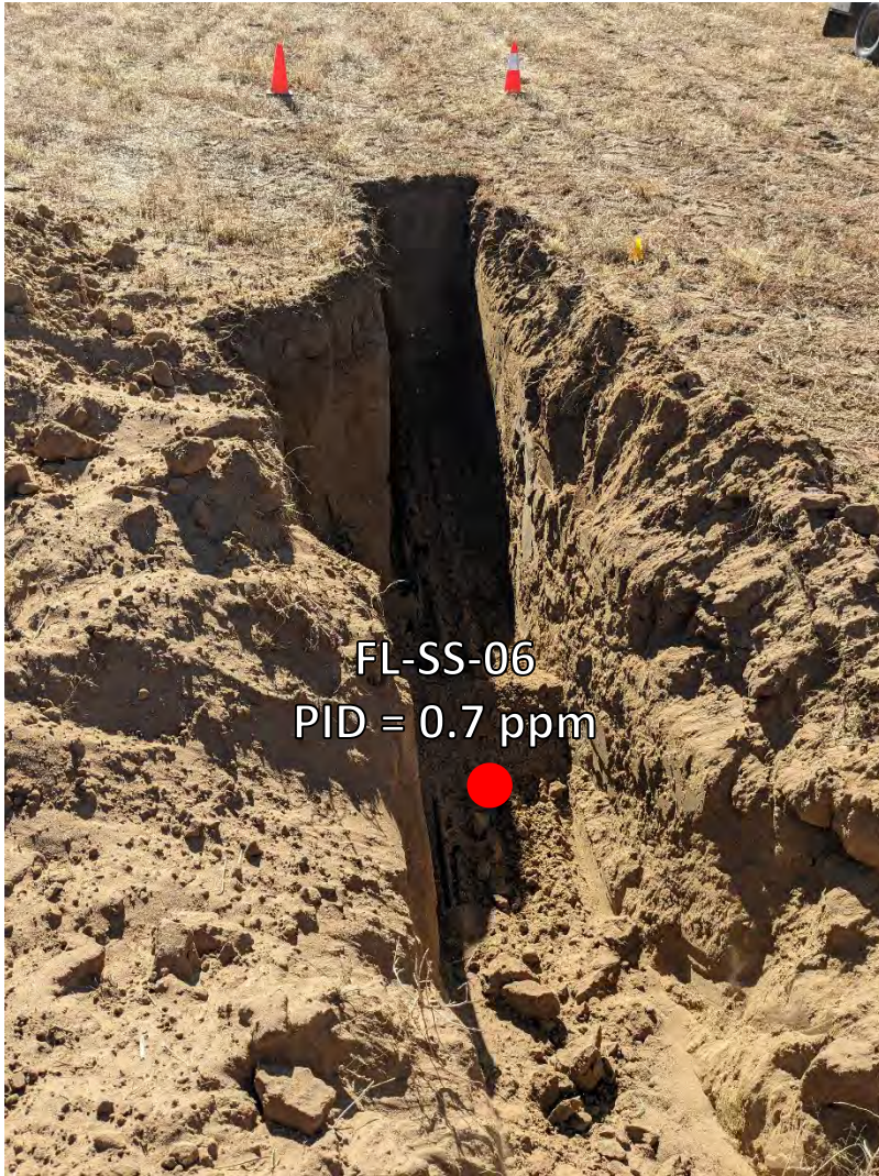
Looking southeast at bellhole/cutpoint No petroleum hydrocarbon staining or odor observed
