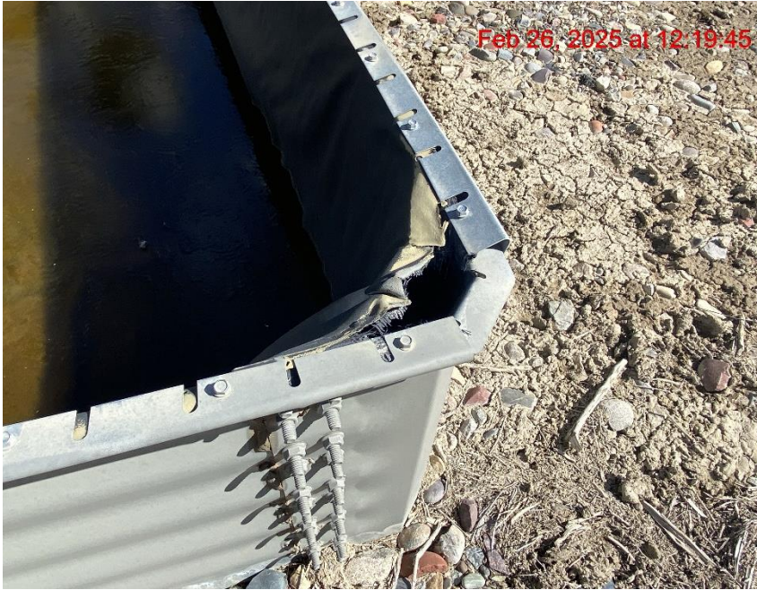
Berm Liner Separating From Containment – Photo #06882
