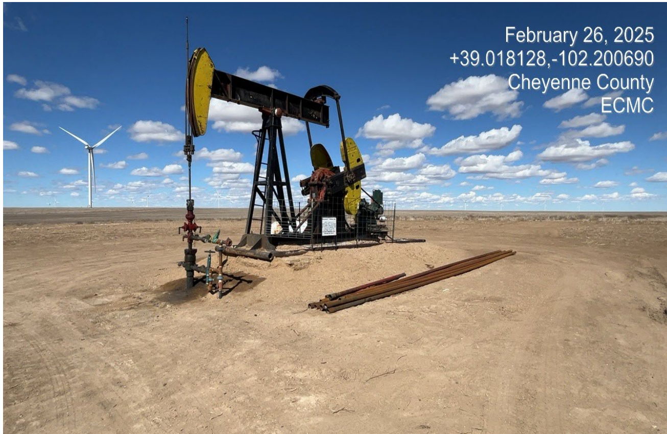
Photo 4. Facing toward the producing well. There are stained soils at the wellhead that must be cleaned up. Previous CA was not completed.
