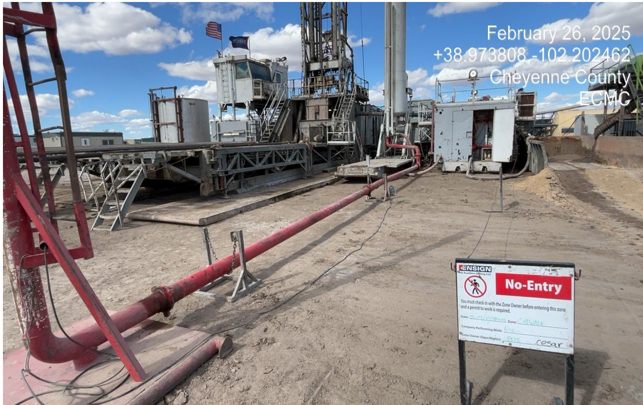
Photo 7. Facing toward the drill rig. There was no liner of other BMPs under the rig to prevent contamination.
