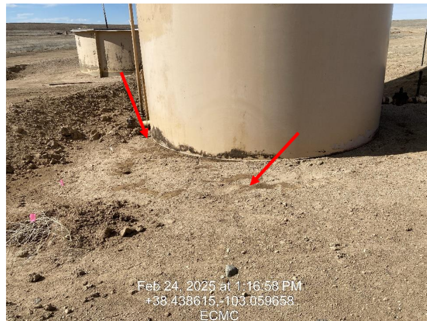
Photo 8 – Impacted soils in tank containment, Spill Id 486875
