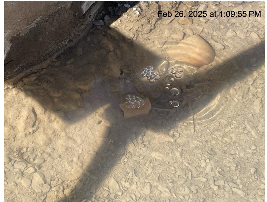
Photo # 9300 Mechanical Condition - Possible wellhead leak /gas bubbling up through water in cellar (GGU Kaufman 22C-30-691)
