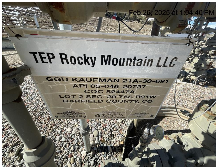
Photo # 9305 Wellhead sign missing required information
