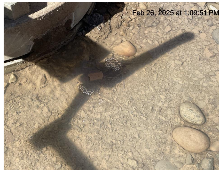
Photo # 9298 Mechanical Condition - Possible wellhead leak /gas bubbling up through water in cellar (GGU Kaufman 22C-30-691)
