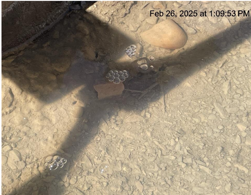
Photo # 9299 Mechanical Condition - Possible wellhead leak /gas bubbling up through water in cellar (GGU Kaufman 22C-30-691)
