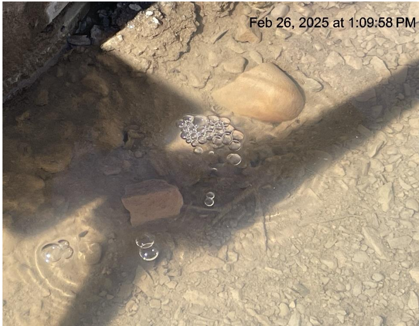
Photo # 9301 Mechanical Condition - Possible wellhead leak /gas bubbling up through water in cellar (GGU Kaufman 22C-30-691)
