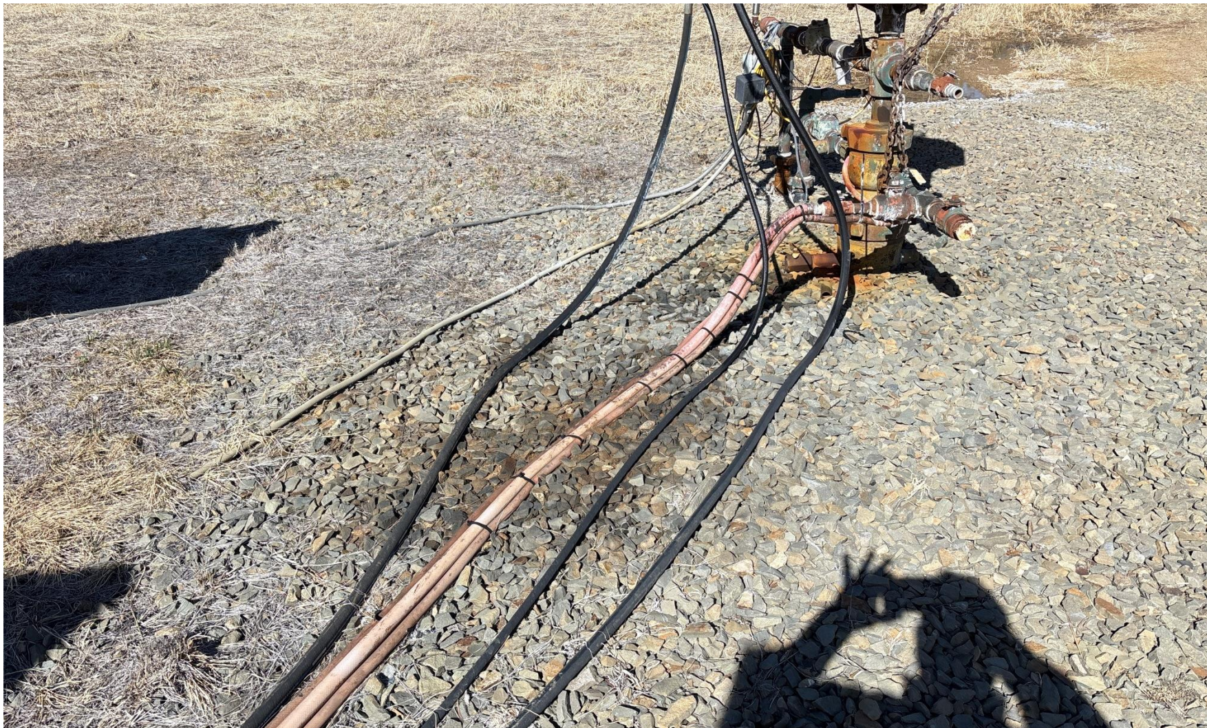
PHOTO 4: THERE IS AN AREA OF IMPACTED SOIL APPEARS TO BE FROM PREVIOUS HYDRO HOSE LEAK THAT APPEARS TO BE FIXED. Conduct maintenance on equipment, cleanup stained material and review self inspection processes. COMPLY WITH RULE 1002,(2).D CA DATE 3-5-2025.
